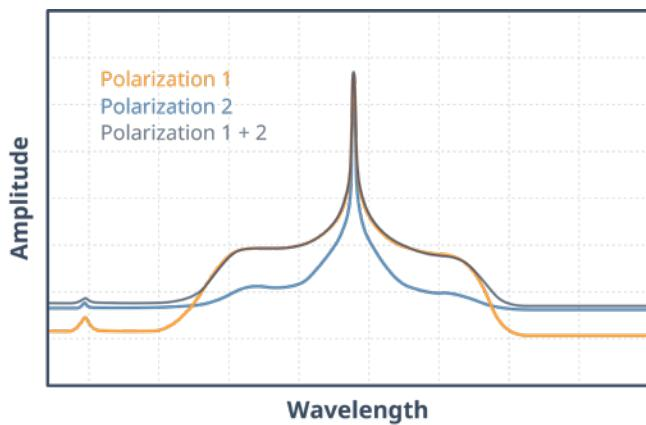
Two polarization channels displayed separately and simultaneously, or combined for polarization independent measurements.
