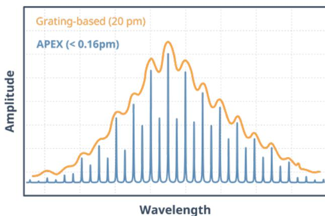
Hundreds of times better resolution than grating-based/monochromator OSA allows to accurately measure the smallest features.
