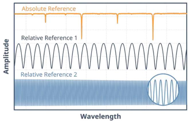
Absolute accuracy of the tunable laser source, maintained using three (3) distinct wavelength references, also allowing the analyzer to be used as a wavelength meter.
