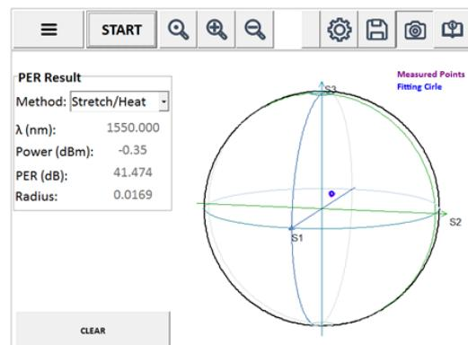
SOP, DOP, and PER measured with high accuracy and allowing fast sampling rates, over a wide range of input optical power. Information displayed as Jones vectors, Poincare sphere, and Stokes parameters.
