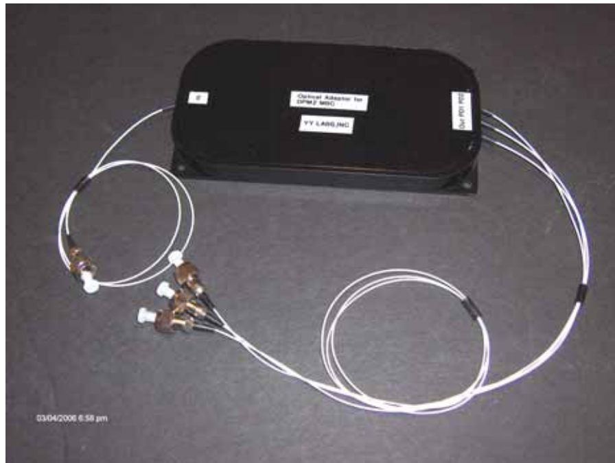
Figure 3. Optical Adaptor for DQPSK MBC
