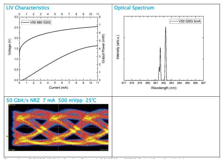
Transmitter: SHF BPG 12104A. Receiver: Tektronix DSA8300 w. 80C15 Optical Sampling Module. **Eye diagrams show intrinsic performance of the chip. No equalization or signal processing was applied.** If the eye-diagram is open at 50Gbaud NRZ without equalization, one can expect good 100Gbit/s PAM4 transmission quality if appropriate PAM driver or/and pre-equalized signal is applied.
