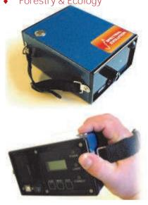
PSR-1100 Spectroradiometers may be ordered with either a 4° FOV lens (shown above) or with a 1m fiber optic. Lightweight rugged compact case, fingertip control trigger, laser sighting and hand strap allow for convenient one-handed operation in the field.
