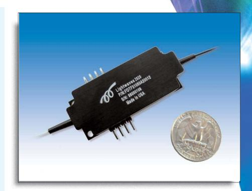
The Lightwaves2020 High-Speed Tunable Filter is a tunable optical filter to choose specified wavelengths over a certain range. The wavelength tuning is achieved by applying a control voltage. The typical wavelength scanning frequency is >1kHz.
