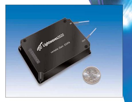
In December, 2009, Lightwaves2020 released one compact variable gain EDFA module with low noise figure. With Lightwaves2020's proprietary Liquid-crystal Variable Optical Attenuator and Thin-film based Gain Flattening Filter, the variable gain ranges from 15dB to 25dB within wide input power range. This makes the module suitable for pre-amplifier, inline, and booster applications. Our products achieve gain deviation  $< \pm 2$ dB & noise figure < 7dB over all operating conditions.
