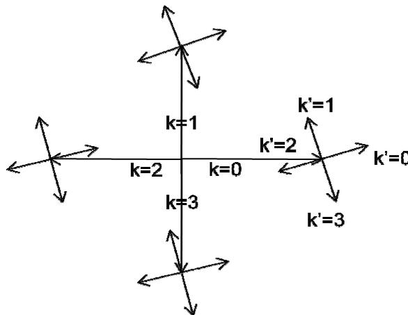
The spacing between the 16 points of the constellation is determined by the splitting ratio ( $R$ ). The orientation of the sub-constellation  $k'$  has to be adjusted, depending on the modulation frequency, with the phase tuning element.
