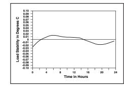
With a typical drift within 0.01°C over a four-hour period, the LDT-5412 out performs similar thermoelectric temperature controllers.
