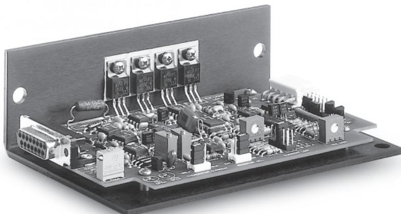
Board-level laser diode current & TE control
