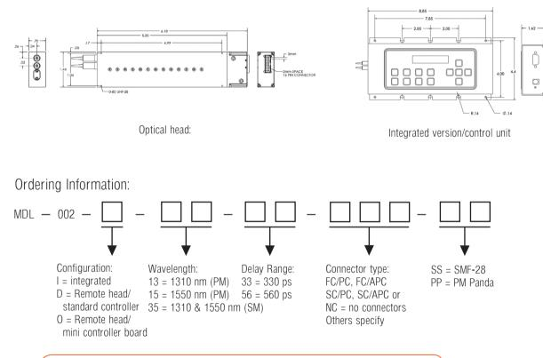
Note: For SM pigtails, the default configuration is 3mm jacketed. For PM pigtails, the default configuration is 900 µm loose tube jacketed.
