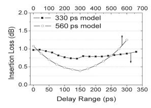
Figure 1. Insertion loss vs. optical delay.
