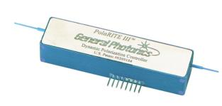
products, the PolaRITE™ III's unique all fiber construction eliminates practically all insertion loss and backreflection. Combined with General Photonics' miniature piezo driver card, it can be controlled either by a digital or analog signal to obtain any desired polarization output from an arbitrary input polarization state.
