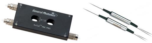
This device can be used either as a polarization beam combiner to combine light beams from two PM input fibers into a single output fiber, or as a polarization beamsplitter to split light from an input fiber into two output fibers of orthogonal polarization states. An important application of this device is polarization division multiplexing or demultiplexing in optical
