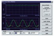
DGD and PSP measurement (Jones Matrix Eigenanalysis) of two 15.75 mm YVO<sub>4</sub> crystals with 45° alignment. Specified DGD=15.90ps, SOPMD=126.46ps<sup>2</sup>, Measured DGD=15.903ps
