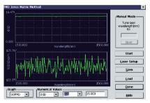
1st and 2nd order PMD measurement (Jones Matrix Eigenanalysis ) of two 15.75 mm YVO<sub>4</sub> crystals with 45° alignment. Specified DGD=15.90ps, SOPMD=126.46ps<sup>2</sup>, Measured DGD=15.903ps, SOPMD=124.03ps<sup>2</sup>
