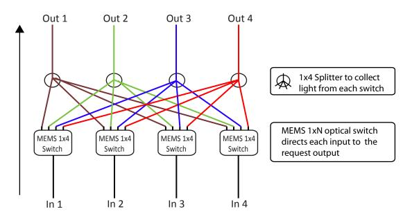
On the Add Side, a series of MEMS 1xN optical switches are used to direct each input to a requested output. Splitters are then used on each output to collect and combine the light from the switches, so that each output can contain any requested combination of inputs.
