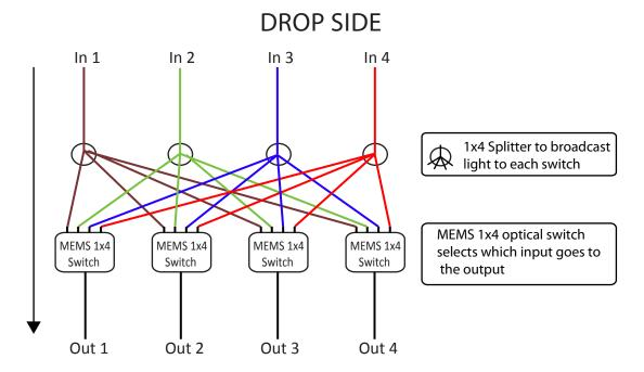
On the Drop Side, splitters are used on each input to broadcast light to a series of MEMS 1xN optical switches, which select which input goes to which output. In this way each output can contain the signal from any requested input.
