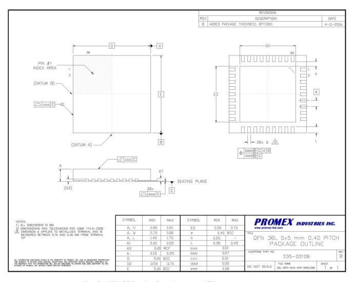
Fig. 2. QFN 36-Pin Package Drawing (All Dimensions in mm)
