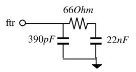
Fig. 2. External Loop Filter
