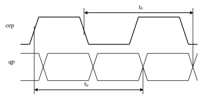
Fig. 3. Output Data to Input Clock Delay
