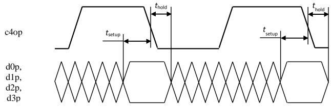
Fig. 2. Input Data Alignment to Output c4 Clock
