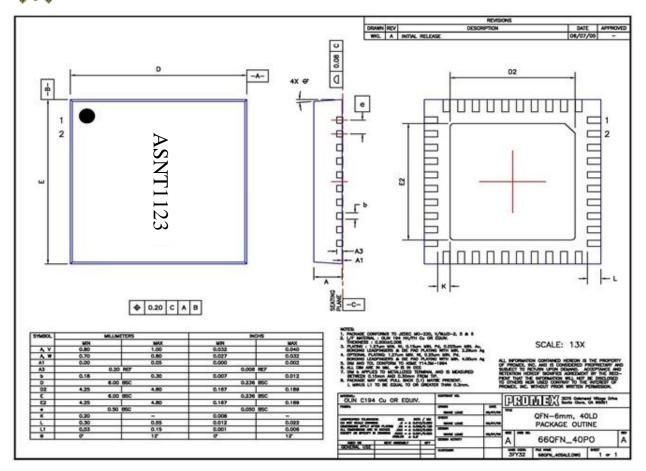
Fig. 4. QFN 40-Pin Package Drawing (All Dimensions in mm)
