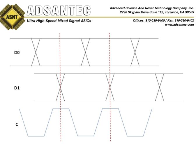
Fig. 2. Input Signal Timing Diagram
