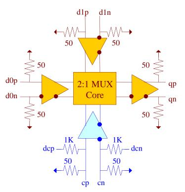
Fig. 1. Functional Block Diagram
