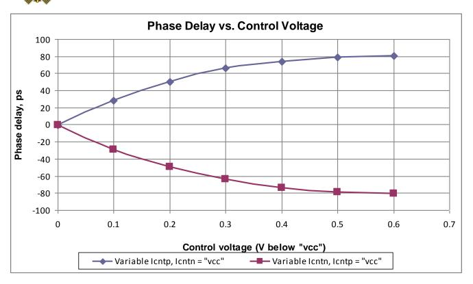
Fig. 2. Delay Control Diagram
