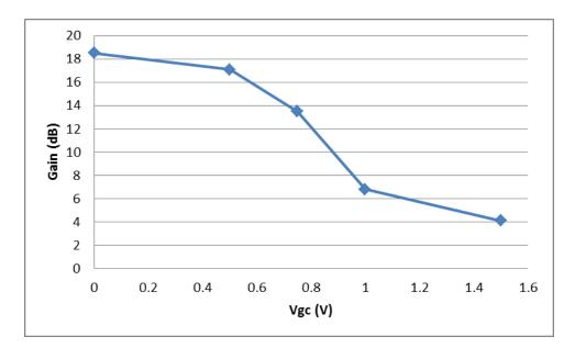
Fig. 2. Single-ended Gain vs. Vgc
