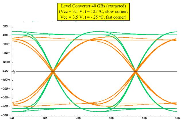
Fig. 3. 40Gbps Simulated Output Eye Diagrams at Different Conditions
