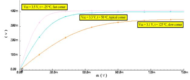
Fig. 2. Simulated DC Transfer Function
