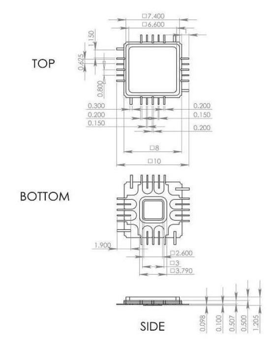
Fig. 4. CQFP 24-Pin Package Drawing (All Dimensions in mm)
