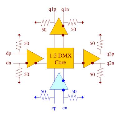
Fig. 1. Functional Block Diagram
