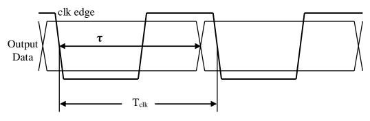
Fig. 2. Output Timing Diagram
